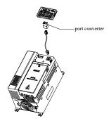
Figure 2-9 Keypad cable link
